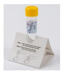
Disposable, one time use tube stand that can be used to hold a **cobas**® PCR Media Tube as sample is being added to the tube
